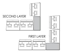
To stay on half bond when installing a 90° outside corner, alternate the direction of the full return corner block on each row. Place masonry adhesive between corner blocks for additional strength.
